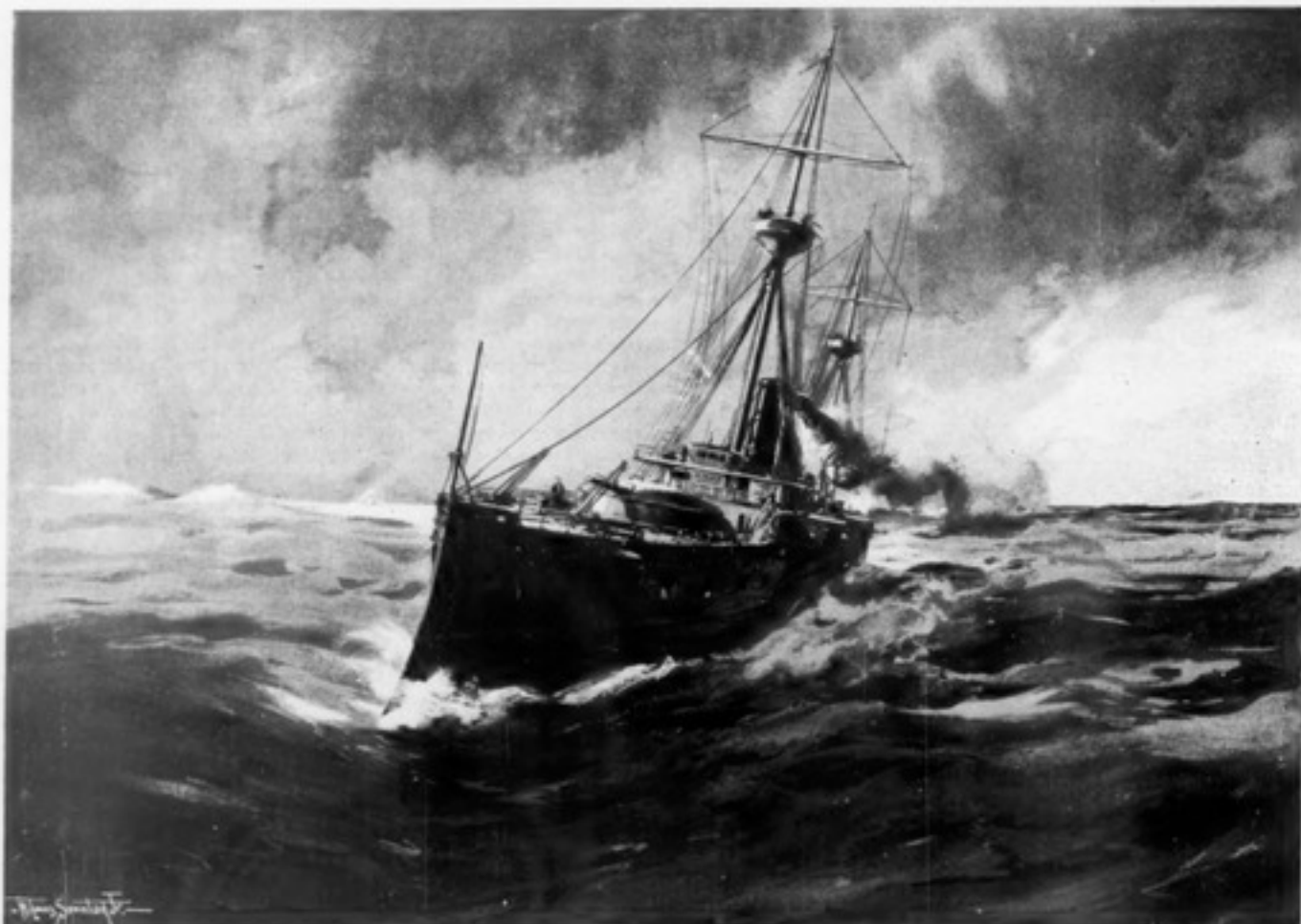
THE "VIZCAYA"—This fine Spanish armored cruiser, now visiting American ports, was completed about four years ago. Her speed is within a knot or two of that of the "New York" or "Brooklyn," but she is much smaller than either of these vessels, the displacements being as follows: "Vizcaya," 4650 tons; "New York," 8500 tons; "Brooklyn," 9915 tons. The armament, also, of the two American cruisers is much the heavier, although in the "Vizcaya's" main battery are two eleven-inch rifles.
